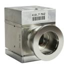
Quantus LP100+ creates a plasma by coupling energy into the gas utilizing a patented planar antenna in the MSC. The antenna is protected by a sapphire window so it is not exposed to the process chamber or gas sample. This provides the LP100+ its unique operating capabilities that allow the sensor to operate in corrosive and aggressive environments. The planar antenna is built using PCB techniques that provide tight tolerances and high performance. The MSC can be replaced in the field.
