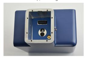
7 Carefully install the new MSC by slowly sliding it down into the housing, without too much force, to ensure the connectors are not damaged and are properly mated. Replace the four (4) set screws using a 2 mm hex driver to secure the MSC in the housing.
