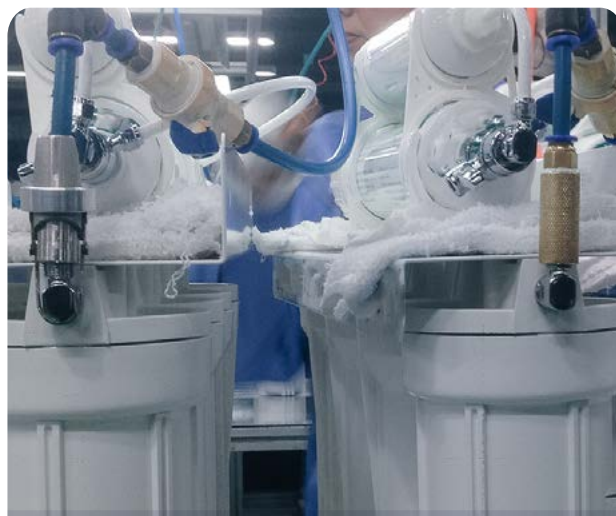
A backlog of units in the testing area needs drying after leak detection with soapy water.
