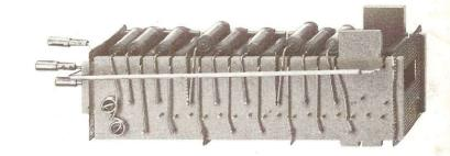
Quadrupole analysers with axially mounted secondary electron multipliers or perpendicular to the mass filter system axis are available. In the latter configuration, a very good signal-noise ratio is obtained, allowing partial pressure measurements of some 10-16 Torr and concentrations determinations in the ppb range.
