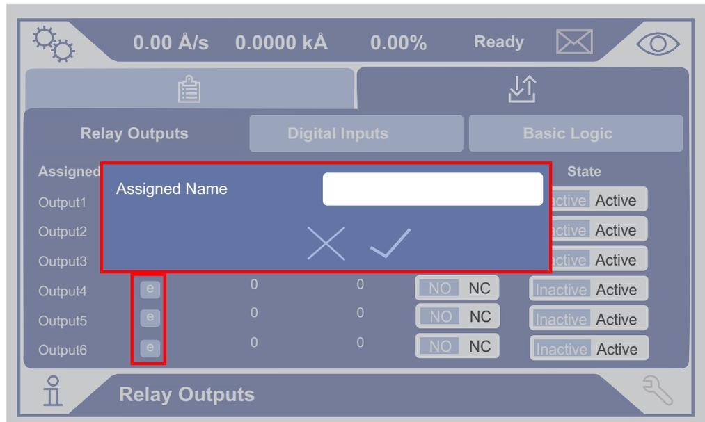
Selecting the **e** next to the relay of interest opens the **Assigned Name** window. This field accepts up to 32 characters.
