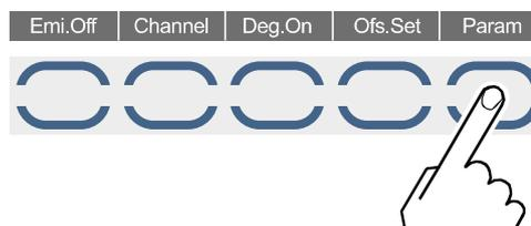
The device changes to the parameter mode. Several submenus are being offered for selection on the display.
