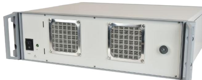
3. Vacuum the stainless-steel dust filters and wipe down the inside of the filter cover front panel grid.
