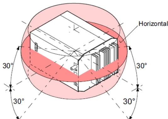
With the holder belonging to the QMH, the QMH can be fastened to the flange. If possible, mount it in such a way that the indicator lights on the back are easily visible.
