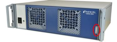
2. Unhook the filter cover front panel grid.
