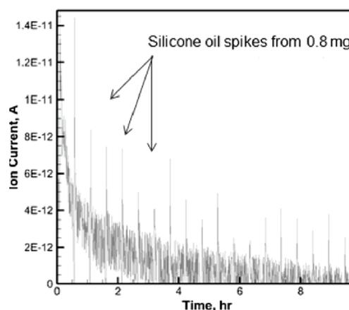
Figure 4: Silicone oil spikes<sup>3</sup>.
