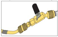
Slowly open the ball valve (B) to charge the system. Close the valve when done.
