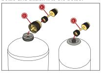
5. With the ball valve (B) in the closed position, connect the refrigerant tank adapter (E) to the T fitting (A).
