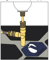
Attach the ball valve (B) to the system.
