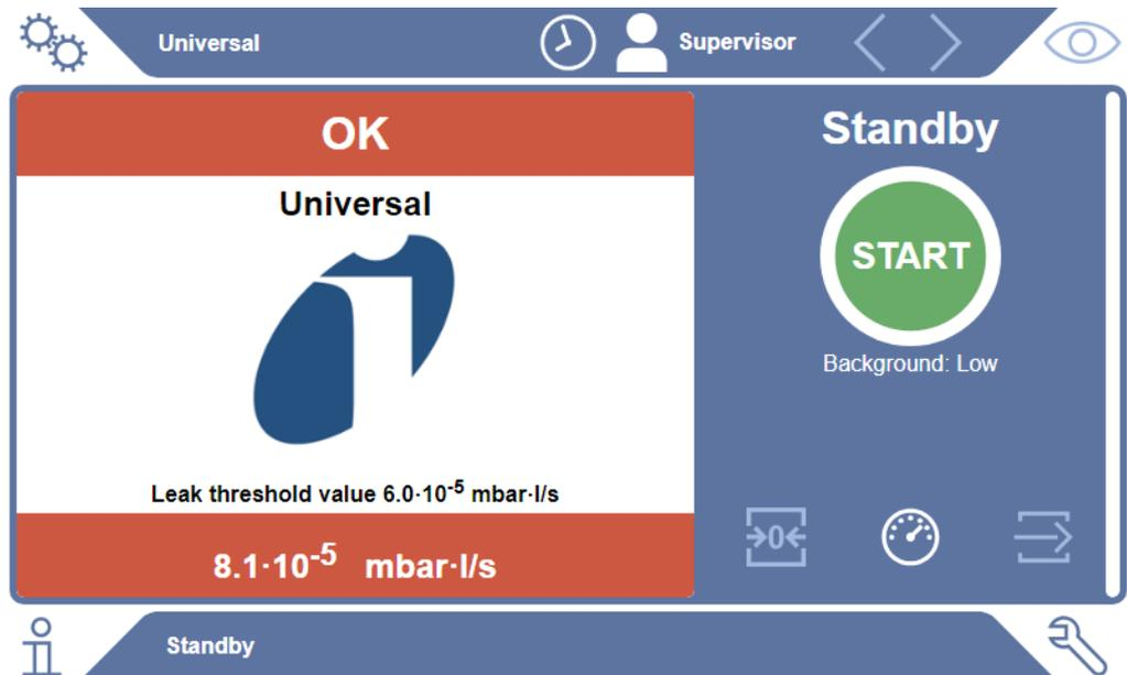
**Measurement result:** If the leak rate is above the setpoint for warning but still below the setpoint for leaks, the measurement result is shown on an orange background. The specification of a setpoint for a warning is optional.
