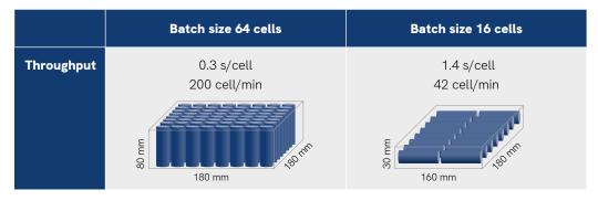
Example batch testing procedure for type 21700 round cells with DMC as solvent: the combination of ideal batch size and high-performance external pump enables high-speed throughput.
