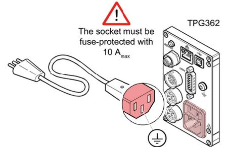
If the unit is installed in a switching cabinet, the mains voltage should be supplied and turned on via a central distributor.
