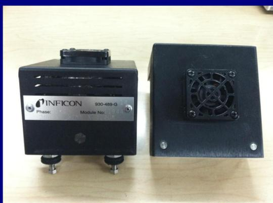
Figure 3: GC Column Module
