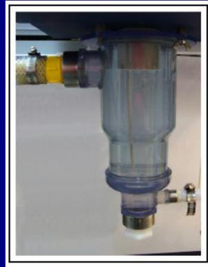
Figure 2: Water sampling vessel with purge tube for argon bubbling
