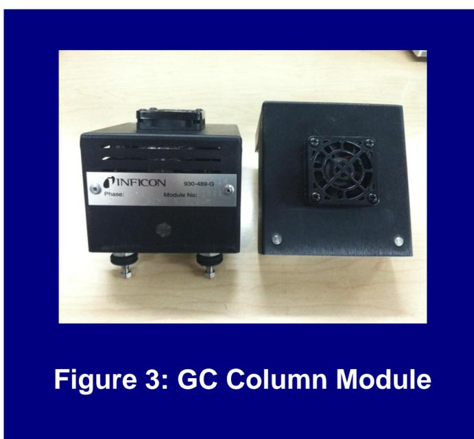
Figure 3: GC Column Module
