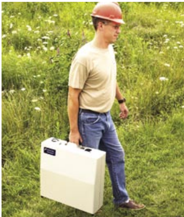
Scenograph CMS100's internal battery and gas supply make it totally portable.
